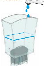
Tilt the water tank back and forth to remove air bubbles from the filter.
