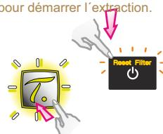
After ~3 seconds, you can release the "Reset filter" button while still holding down the button.
